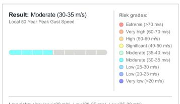
Low risks: Very low (<20 m/s), Low (20-25 m/s), Low (25-30 m/s) Medium risks: Moderate (30-35 m/s), Moderate (35-40 m/s), Significant (40-50 m/s)
